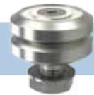
Hepco VACSS Vacuum & High Temperature Bearings are made entirely from stainless steel parts and are lubricated internally for life using Krytox LVP grease. They are suitable for use in high vacuum, at temperatures from -15°C to +210°C, and in the presence of oxygen. They are widely used in applications including semiconductor wafer manufacture, aerospace components, vapour deposition processes, LCD panel and plasma display manufacture and in vacuum evaporation equipment.
