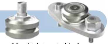
Hepco LTSS Low Temperature Bearings are lubricated internally for life using AeroShell Grease 22 which is suitable for use at temperatures from -50°C to +150°C. This lubricant enables use in much colder conditions than the VACSS bearings, opening up applications in cold stores and specialised freeze dry equipment.
