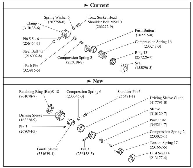
2) Slider and the relevant parts have been changed as shown below.
