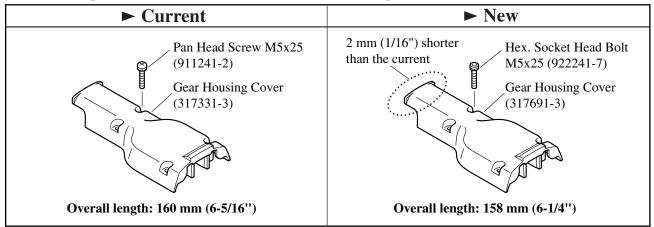
5) Gear housing complete has been changed as shown below.
